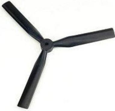
The majority of propellers used in the radio control flying hobby have two blades but props with three or even four blades are available.
