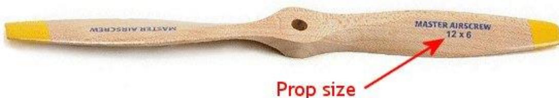
The first number is the **diameter** of the imaginary disc ('arc') created by the spinning prop *i.e.* the length of prop from tip to tip. The second number is the **pitch** and this is the harder of the two to understand – but we'll give it a go...
