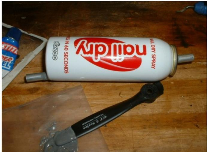
Attach the muffler to the silencer using silicon tubing or a silicon exhaust deflector from local model shops.
