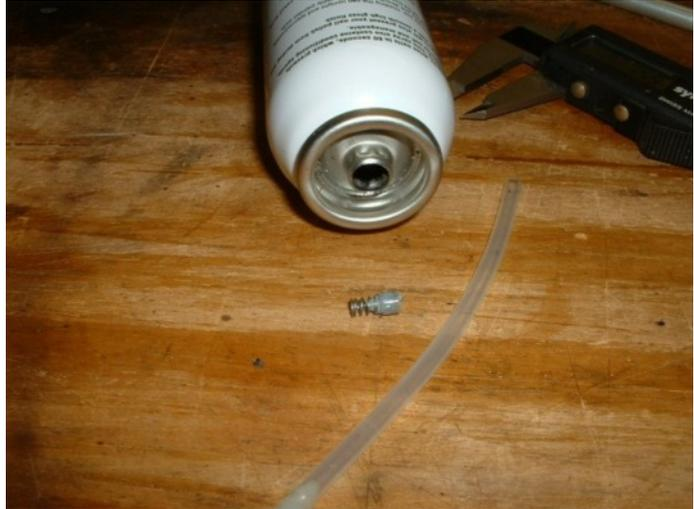
Next, working from bottom end of can, centre-punch the bottom (curved) face, half the dia. of the tube to be fitted from the edge. This will be the lowest point of the muffler and is the position the exhaust stub will be.
