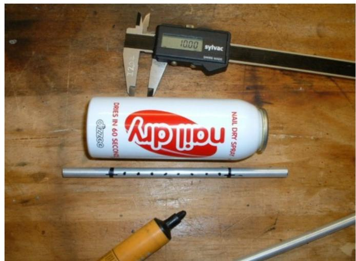
The 4mm pepper pot holes in the pipe are drilled THROUGH @ 10mm spacing. Then turn pipe 90deg and drill THROUGH and between 1<sup>st</sup> drilling. Continue drilling to 75% length of muffler can. A small 2mm oil drain hole is drilled in one end of the pipe in a position to sit just inside the muffler can. This is to enable any oil and water collected in the muffler, to exit via the outlet stub.
